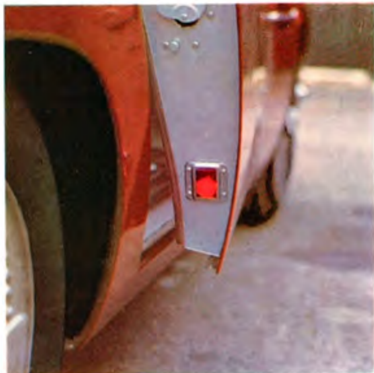
Trailing edges of the doors carry red warning lights.
